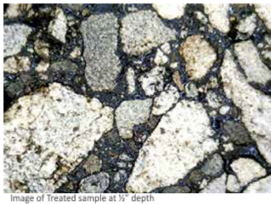
Figure 10b. Images at 40x magnification of the voids and FT-IR scan of treated asphalt concrete samples at ½” depth (Cochran Engineering, Inc., Union, MO).
