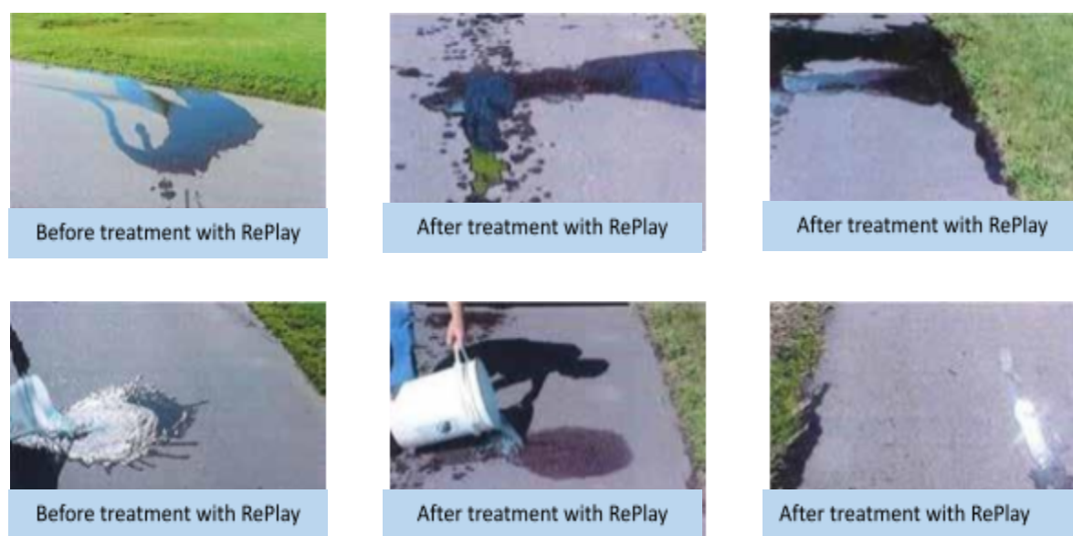
Figure 4. Runoff experiments on an asphalt driveway before and after treatment with RePlay.
