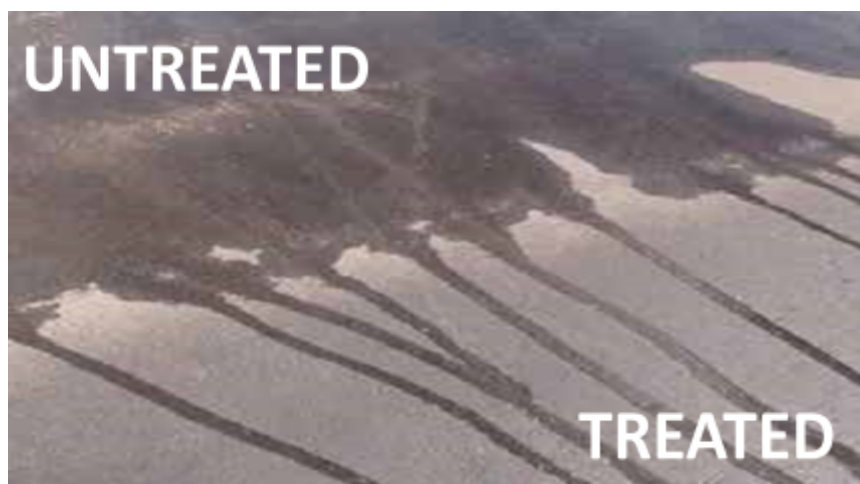
Figure 5. Fast removal of runoff water on asphalt pavement surface treated with RePlay (BPS 2014).
